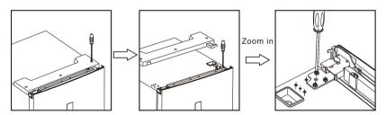
3. Take off the upper door, take out the screw from the middle hinge by cross screwdriver, then take off the lower door.
