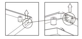
13. Lastly, using the screw to fix the top cover.
